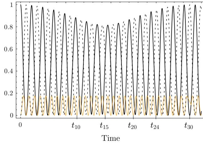
**Figure 6.** Plot of the populations for each state as a function of time for the frequency  $\frac{3\omega_0}{\omega_1} = -\frac{1}{30}$  and  $a \simeq -1.05597$ . The zeroes of the second state population fix the times for the appearance of the quantum gates. In this case we have 30 different gates. The solid line represents the probability for state 1, the dashed line for state 2 and the dotted line for state 3.
