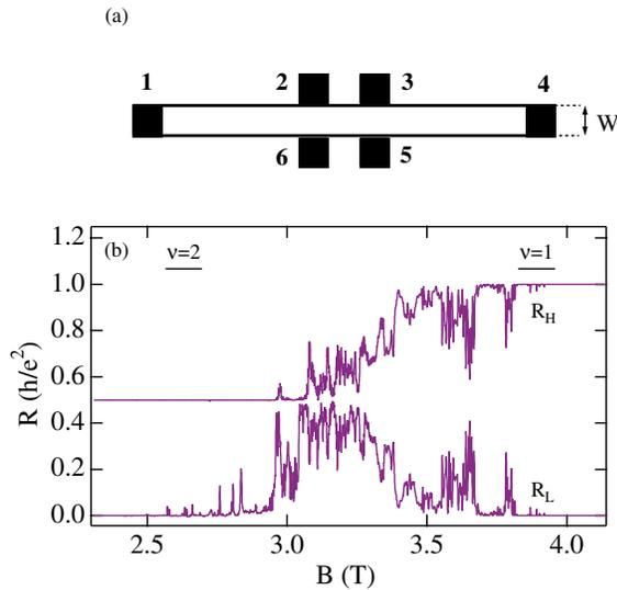
FIG. 1 (color). (a) Geometry of the Hall-bar samples. The black areas represent Au-Ge-Ni contacts. The separation of the current and voltage contacts are  $12 \times W$  and  $2 \times W$ , respectively. (b)  $R_L$  and  $R_H$  vs  $B$  of the  $2 \mu\text{m}$  Hall bar in the vicinity of the  $\nu = 2-1$  transition,  $T = 10 \text{ mK}$ .
