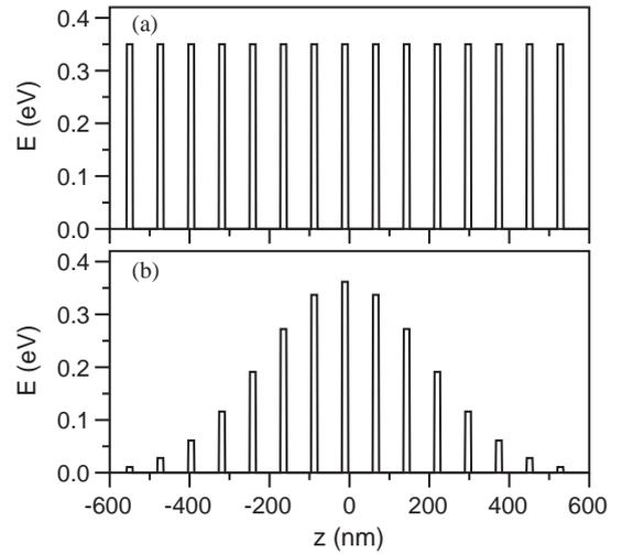
Fig. 1. Schematic diagram of the conduction-band edge profiles of (a) uniform and (b) Gaussian SLs.
