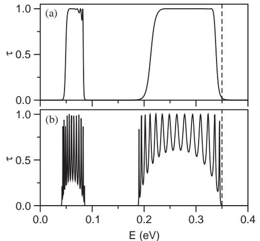
Fig. 2. Transmission probability  $\tau$  as a function of energy  $E$  for (a) Gaussian and (b) uniform SLs with the same number of barriers and layers widths. Dashed lines indicated the energy of the highest barriers. Notice that  $\tau$  is almost constant and equal to unity for the GSL while the usual oscillatory behaviour is observed in the uniform SL.
