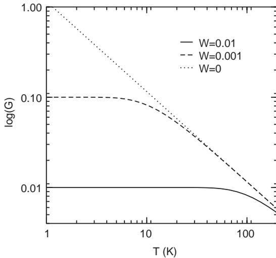
Fig. 6. Conductance  $G$  as function of temperature for several values of the width  $W$  of the ad hoc  $\tau$ , shown in the inset of Fig. 5. The value of  $\mu$  in (c) is  $\mu = 0.10005$  meV and we checked that the results are not modified for any value of  $\mu$  in the vicinity of the transition. The case  $W = 0$  corresponds to the step function. Notice that the smaller the width  $W$  the smaller the size of the plateaus.
