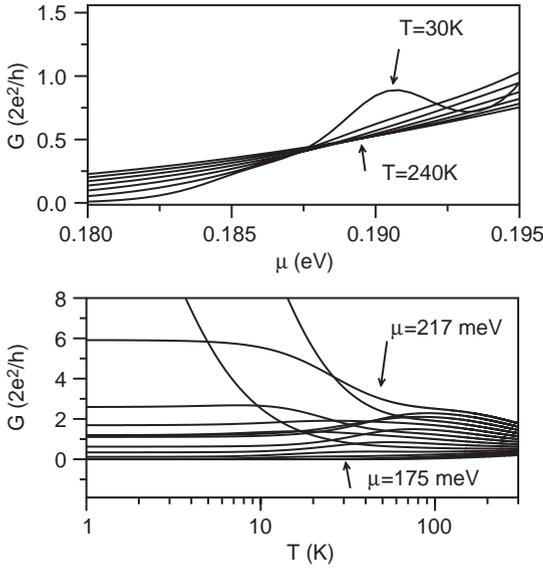
Fig. 4. Conductance  $G$  of the uniform SL as a function of the chemical potential  $\mu$  (upper panel) for several values of the temperature (between  $T=240$  and  $30$  K) and as a function of temperature (lower panel) for several values of  $\mu$  (between  $\mu = 217$  and  $175$  meV). Notice the completely different behaviour as compared to Fig. 3 and the absence of plateaus.
