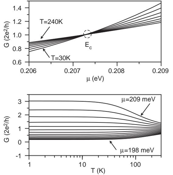
Fig. 3. Upper panel; Conductance of the GSL as a function of the chemical potential  $\mu$  for several values of the temperature between  $T=240$  and  $30$  K. The circle marks the crossing point that allows us to define a critical energy  $E_c = 207.3$  meV. The lower panel shows the conductance  $G$  as a function of temperature for values of  $\mu$  above and below  $E_c$  (between  $\mu=209$  and  $198$  meV). Notice the plateaus in the vicinity of  $E_c$ .
