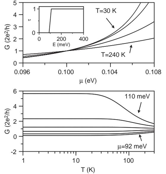
Fig. 5. Conductance  $G$  as a function of the chemical potential  $\mu$  for several values of the temperature ( $T$  between  $30$  and  $240$  K from top to bottom of the upper panel) and as a function of temperature for several values of  $\mu$  ( $\mu$  between  $92$  and  $110$  meV from bottom to top of the lower panel). The inset shows the ad hoc  $\tau$  function used to compute  $G$ .
