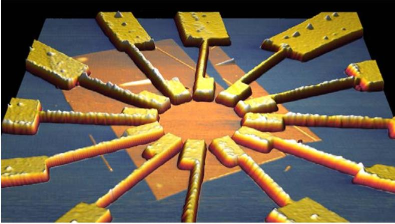
Figure 1: Atomic force microscopy image of a TiS<sub>3</sub> device with electrodes arranged at different angles to probe the in-plane anisotropy.
